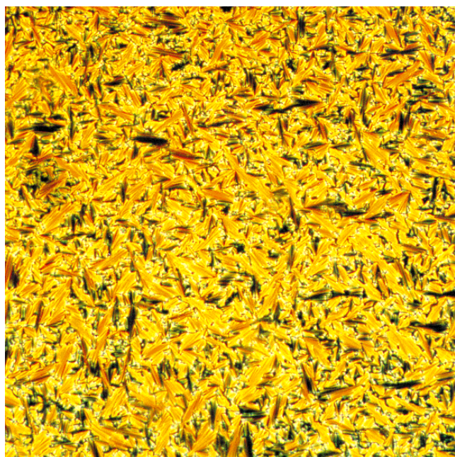
Figure 4. Top: Optical texture of 6 at 120 °C (crossed polarizers, enlargement 200 ×); bottom: Optical texture of 12 at 130 °C (crossed polarizers, enlargement 200 ×).
